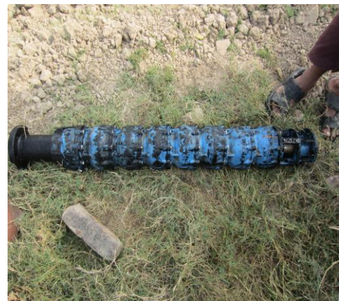
Old defective Motor pump
